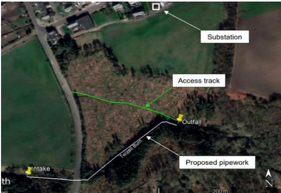
Twizel Burn hydro-power feasibility study
